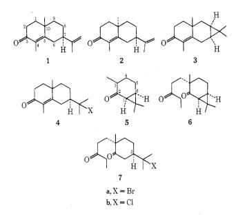
convenient stereospecific synthesis of 1 which employs a similar concept and utilizes (-)-2-carone (5), which is readily available from (+)-dihydrocarvone,<sup>6</sup> as the starting material.
